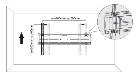
Adjust the adapter brackets to fit the hole pattern of your display. Then tighten all screws with an Allen key. **NOTE:** Verify the proper alignment of all holes.
