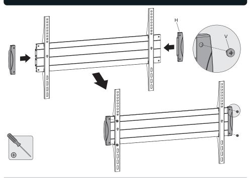
Attach the two plastic covers to both ends of the plate using the appropriate screws. Tighten all screw using a suitable screwdriver.
